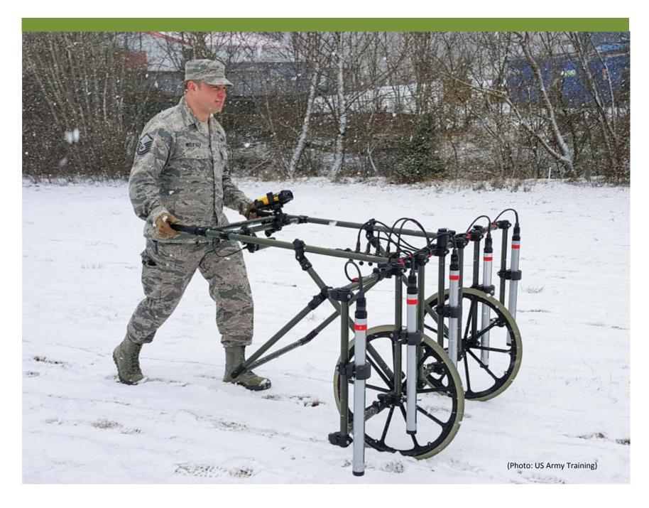
For improved productivity and enhanced data quality EBINGER offers MAGNEX® 120 multi-system for digital surveys. The wheeled system TR01-05 offers space for 5 probes. Probe distance and height over the ground can be adjusted accordingly. Various wheels offer the use in difficult terrain.
