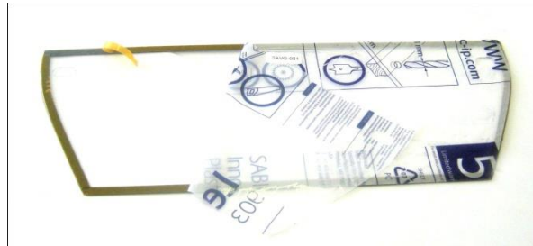
One layer of protective foil removed prior to fitting
