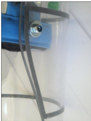
The AVG is fitted to the main visor with securing bolts that are only partially tightened.
